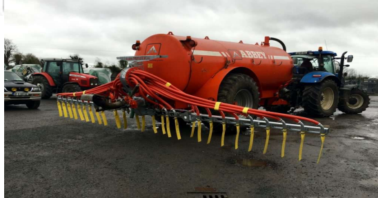
Figure 4: Slurry application methods (a) on top of herbage and over entire spreading width with splash plate method, (b) in lines on top of herbage with band-spreader method, (c) in lines below herbage, but above the soil surface, with the trailingshoe method, and (d) below the soil surface (approximately 5 cm)
